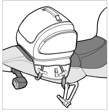
Unzip the pockets on the side flaps of the Tail Pack, pull out the Bungee cords and hooks. Thread them through the loops on the side flaps.
