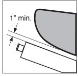
Check the saddlebags are positioned with a minimum of 1" clearence above exhaust pipe (see diagram to left).
