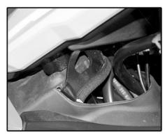
Locate the factory metal bracket positioned underneath the steering head. It might be necessary to turn the handlebars to full lock to access easier.
