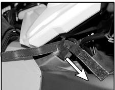
Pass the webbing strap at the front of the bag with Velcro through the metal bracket and pull snug. Repeat on opposite side.
