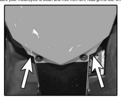
Raise the seat and locate the point where the clips will attach to the tank cowl.
