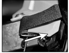
Slide the clip under the plastic cowl as shown Pull webbing forward and make sung. Repeat on opposite side and lower the seat. Be sure the seat is locked in place before proceeding.
