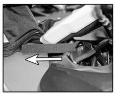
Lay the webbing strap back on itself joining the Velcro patches and securing the bag in place. Repeat on opposite side.
