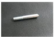
With the body removed, thread in by hand your spot tool. Make sure you have the spot tool screwed in enough to clear the body on the inside.
