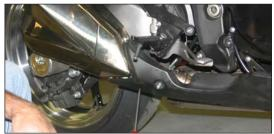
6. Remove right side exhaust muffler.
